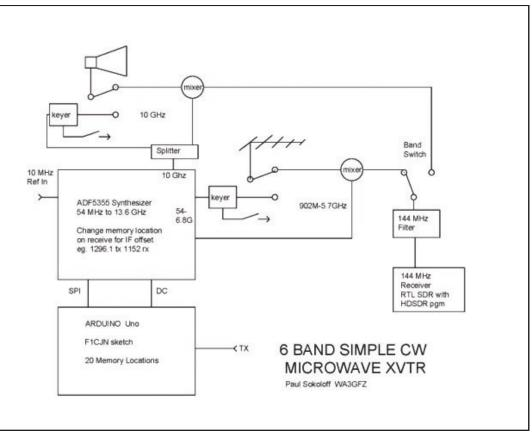
Arduino controller for transmit and the down button to get us back to the receive LO frequency. Keeping it simple, the T/R relay is used for keying.
