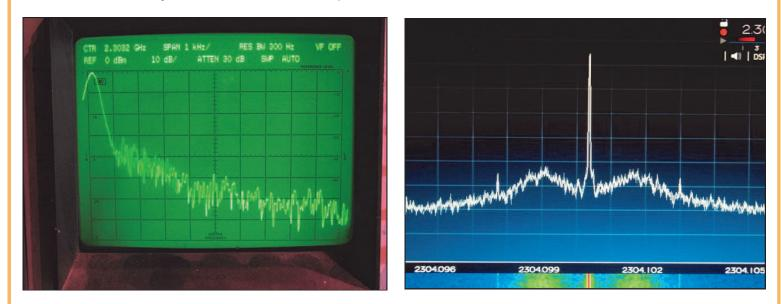
The power supplies on these boards are their downfall. They cause the bad phase noise. There are modifications that can improve this, but for my application it is fine. The other issue is poor RF isolation of the relays. Some signal does leak through when not transmitting. One solution could be to modify the software to look at the key and switch to the TX frequency only when keyed.
